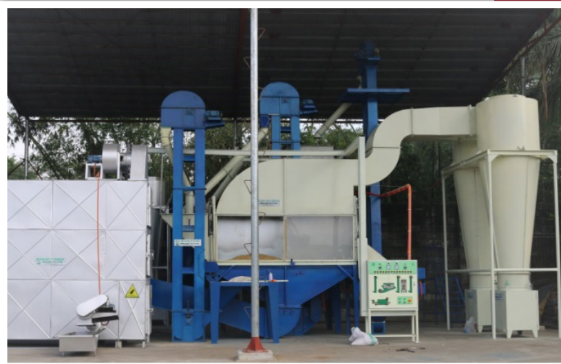
Fluidized Bed Dryer set up in Nueva Vizcaya.
